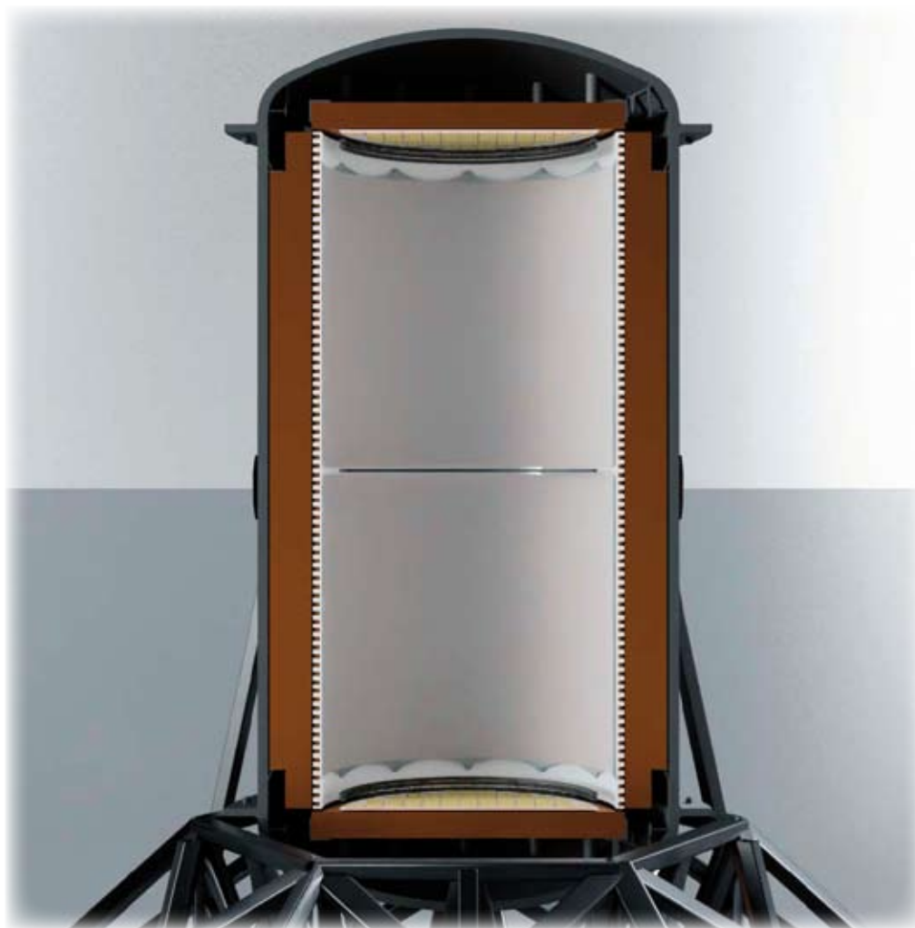
Image of the NEXT-HD detector in its vertical orientation. NEXT-HD will have two identical sensor planes with SiPMs mounted on ultrapure substrates.
