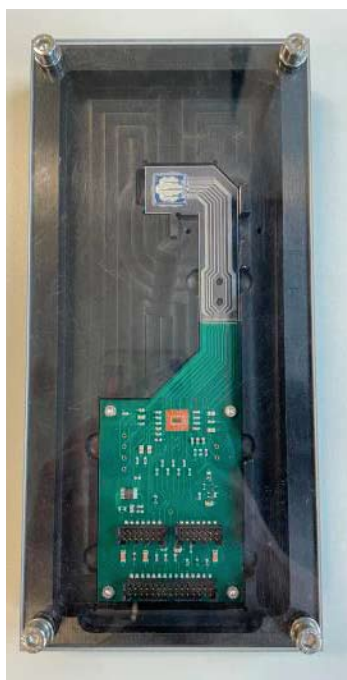
Fig: Split PCB with a "head" made from radio pure silicon.
