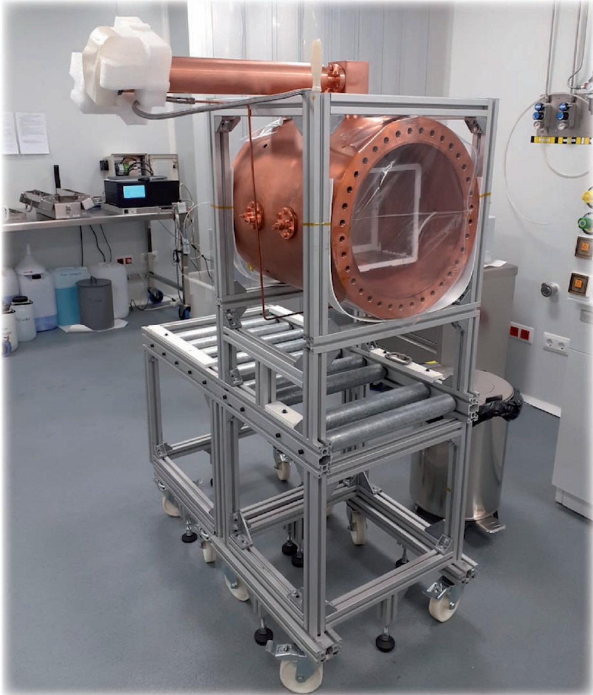
TREX-DM shielding inside the Clean Room
