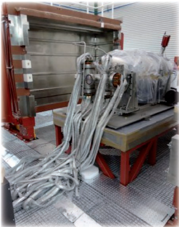
The tracking plane feedthrough manifold at NEXT-White
