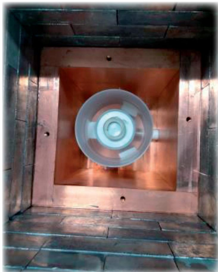
*Sample analyzed in the rediopurity measurements using HPGe of LSC*
