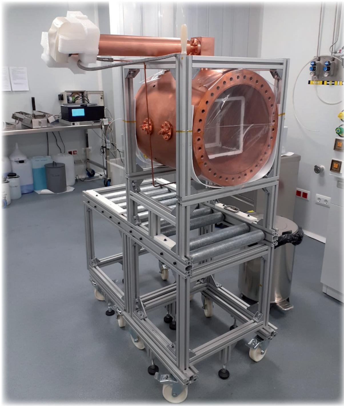
TREX-DM shielding inside the Clean Room
