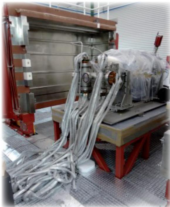
*The tracking plane feedthrough manifold at NEXT-White*
