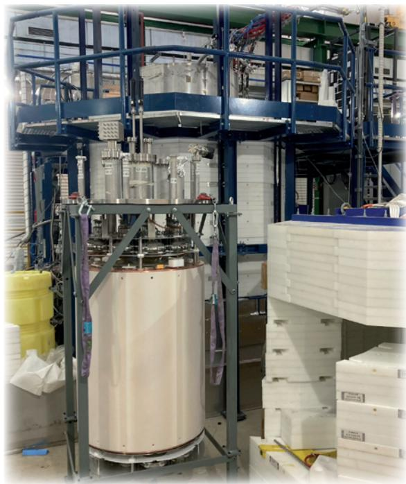
DArT at ArDM is a proof-of-concept for a facility to determine the radio-purity of argon with high precision. The goal is to measure the intrinsic contamination by  $^{39}\text{Ar}$  and  $^{85}\text{Kr}$ , of argon samples purified at the distillation column (Aria), and/or recuperated from the  $\text{CO}_2$  gas well (Uraria) of the Kinder-Morgan plant,
