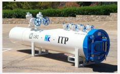
These prototypes are tested in high pressure water environments, what is called a 'hydrostatic test', in order to be validated by the Hyper-Kamiokande collaboration.
