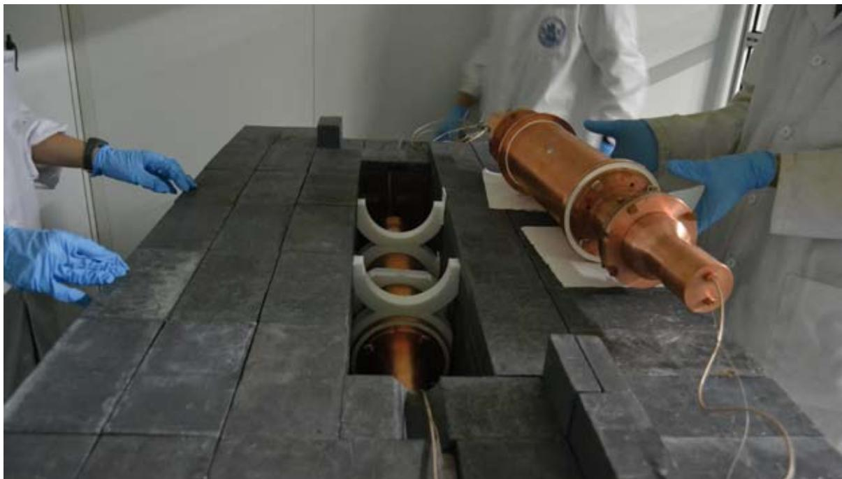
anti-radon box(continuously flushed with radon-free nitrogen gas), active muon veto system made up of 16 plastic scintillators designed to cover top and sides of the whole ANAIS set-up and 40 cm of neutron moderator (a combination of water tanks and polyethylene blocks). In the design of the muon veto system we followed a tagging strategy instead of a hardware vetoing.
