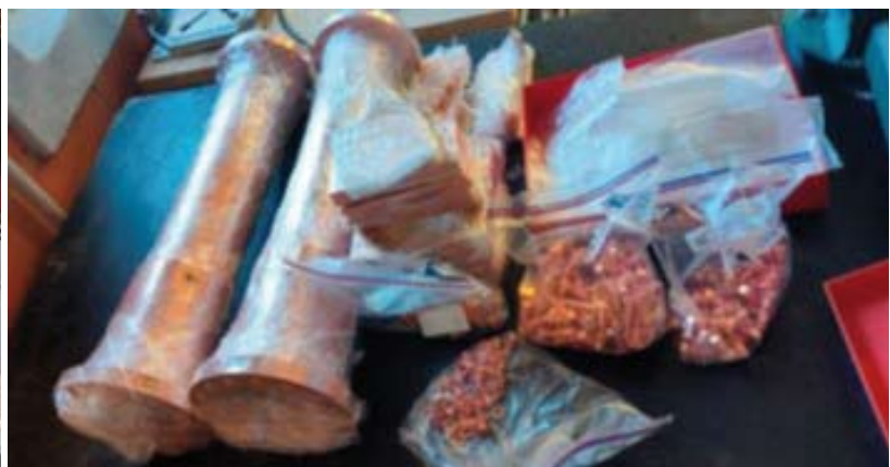
Chemical cleaning performed at Unizar (left) and cleaned copper pieces preserved (right).
