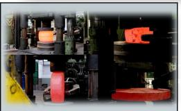
**Ton-scale forged Copper** The internal shielding of the NEXT-100 vessel includes a thick dish of ultrapure copper, forged to resist the big change of pressure between the interior of the vessel and PMT zone. Fresh Copper was welded, forged, machined and cleaned before at LSC.
