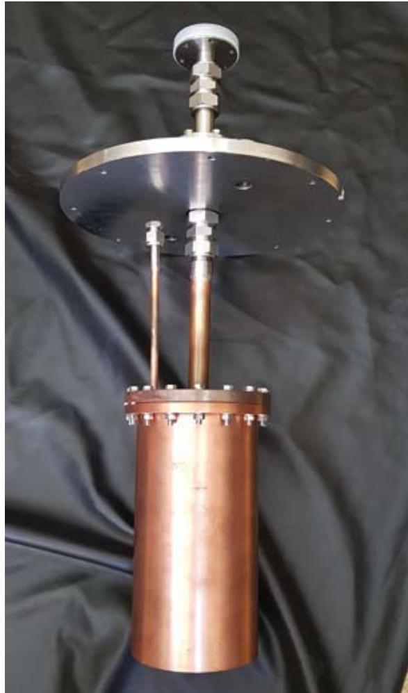
*(Left) Sketch of the inner structure of DArT. (Right) Picture of the actual detector. The short stainless steel pipes are used in the cryogenic tests, and will be replaced by longer tubes in the final setup.*
