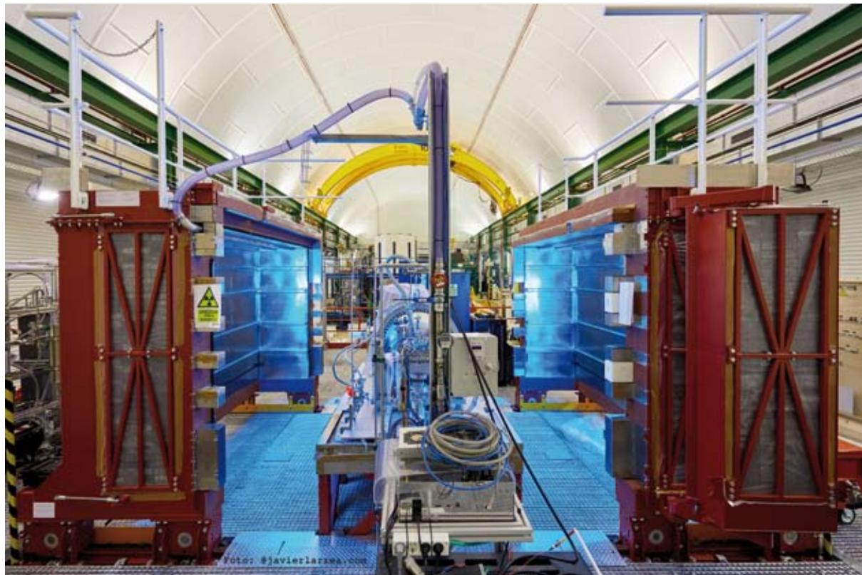
constructed from the titanium-stabilized stainless-steel alloy  $^{316}\text{Ti}$ . The vessel sits on top of a seismic table, and a lead shield that can be mechanically opened and closed surrounds the vessel. The vessel is connected to a gas system through which the xenon gas is continuously purified via the use of a hot getter. The entire experimental area, including gas system, electronics, pressure vessel, and seismic table, are stationed on an elevated tramez platform at LSC.
