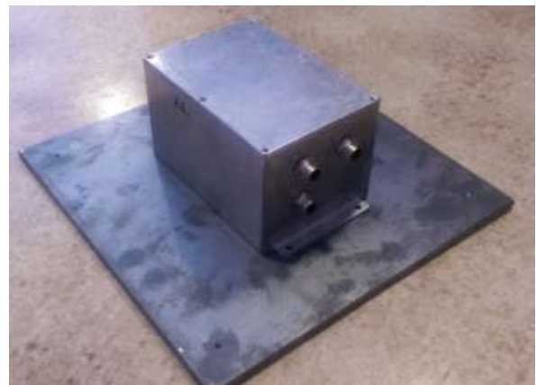
Fig.13.1: The seismic sensor mounted on a steel plate. The top two connectors are used for data communication, while the bottom one is used to provide power..
