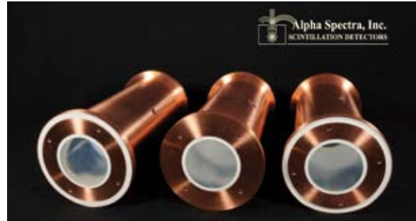
Fig. 5.1. Last three ANAIS AS modules, 12.5 kg of NaI(Tl) each, received in March 2017 (D6, D7 and D8), completing the 3x3 matrix of detectors ANAIS112 consists of.
