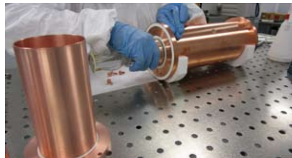
Fig. 5.2. Coupling of the PMTs to D6, D7 and D8 modules at LSC clean room, March 2017.
