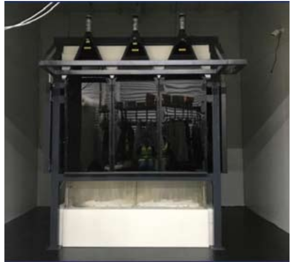
Fig. 5.6. ANAIS112 set-up before completing the neutron shielding. Plastic scintillators vetoes, installed in May 2017, can be seen.
