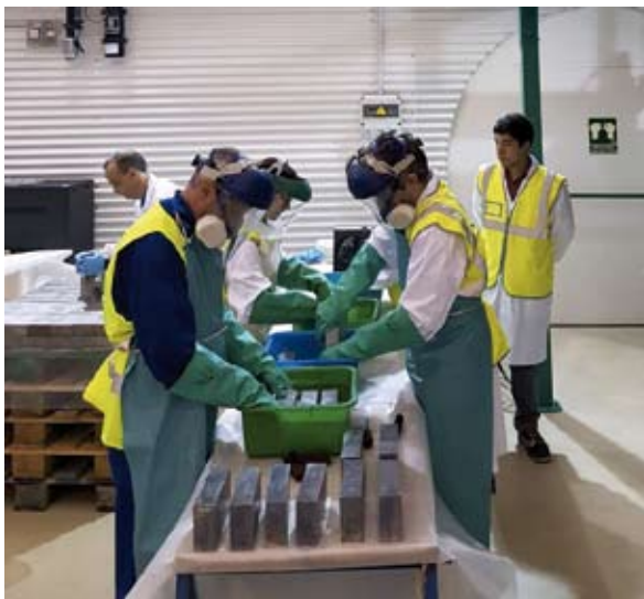
Fig. 2.1: Cleaning of lead in preparation for the installation of TREX-DM in Hall A
