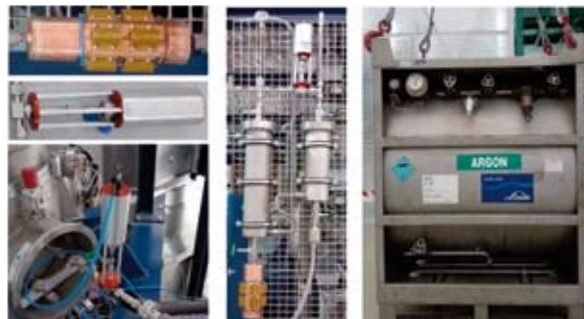
Figure 6.2: Evaporator and motorised valves (left), filter components (middle) and LAr tank (right), used for the filling of nearly 1.5 tonnes of LAr of the ArDM target.
