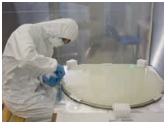
Fig. 6.4: Assembly of the extraction grid and the ITO-TPB-coated PMMA anode window in a clean tent built in Hall A of LSC (July 2016).
