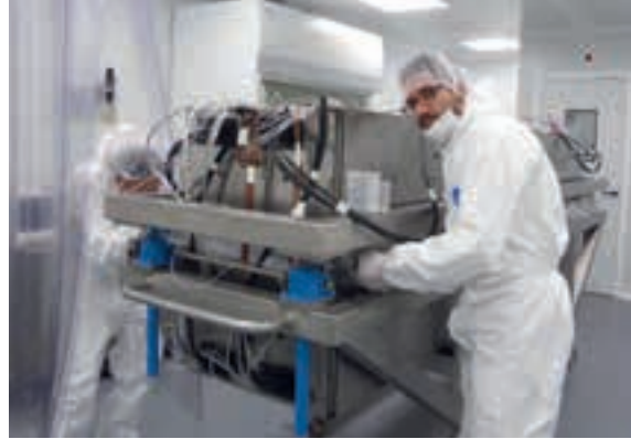
Fig 8.2: Installation of LAPP foils in one of the BiPo-3 modules.
