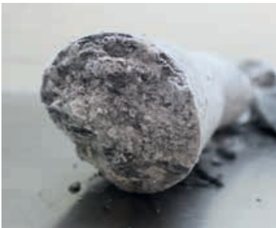
Fig. 12.2: Picture of a fragmented core
