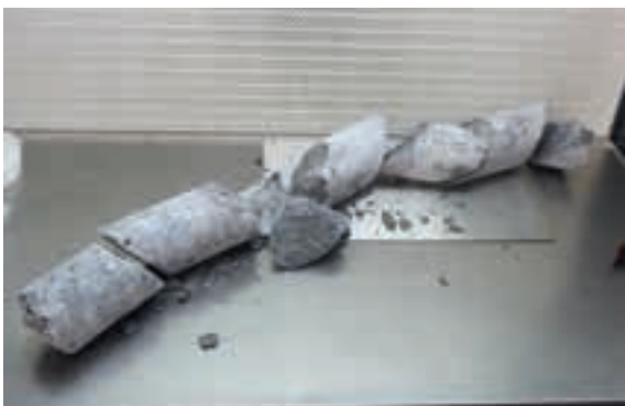
Fig. 2.1: Example of core (5A) fragmented in pieces
