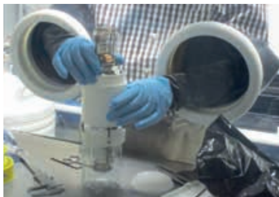
Fig. 5.4: Mounting a 1 kg piece NaI(Tl) in the glove box at the University of Zaragoza.
