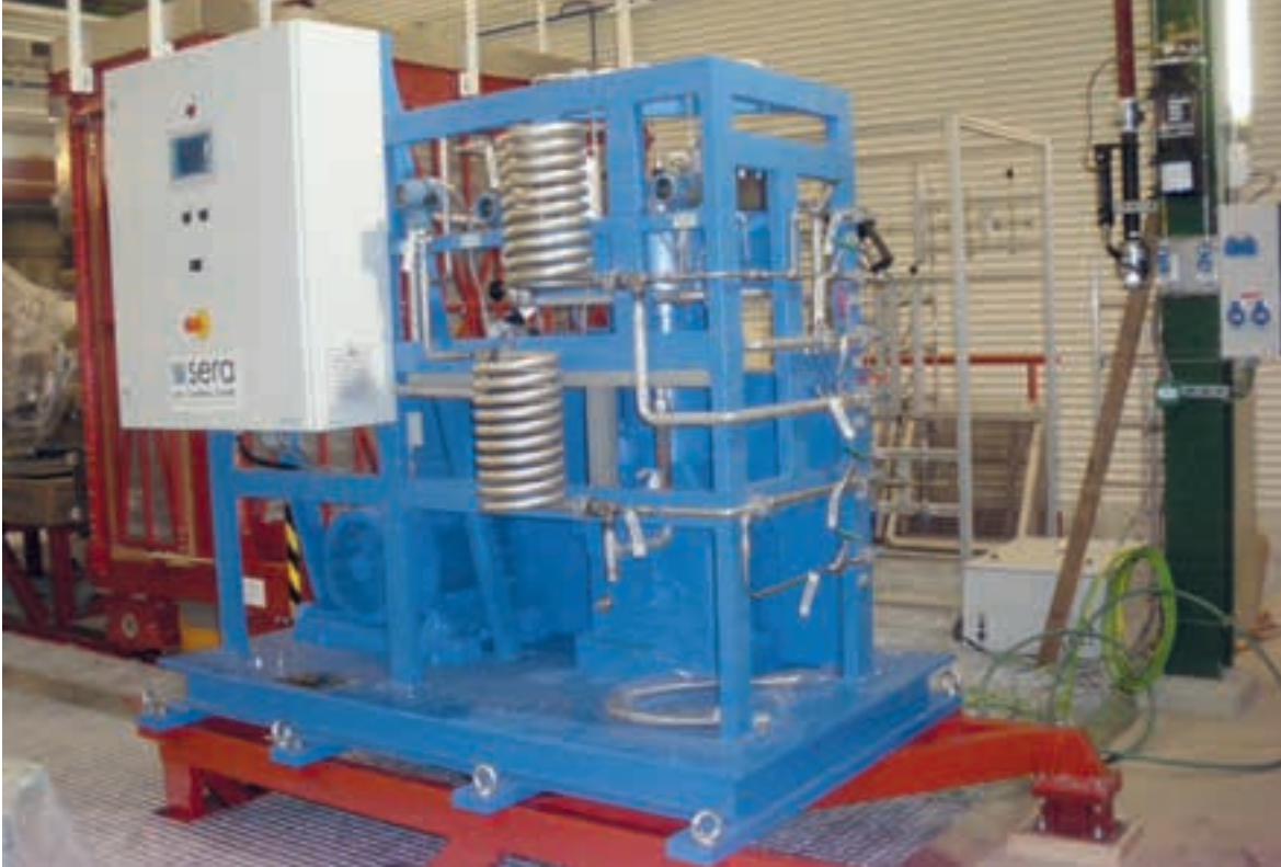
Figure 6.2: The compressor chosen for NEXT, manufactured by the SERA company, in Germany. The pump is made with metal-to-metal seals on all the wetted surfaces. The gas is moved through the system by a triple stainless steel diaphragm, ensuring a negligible probability of catastrophic failure (gas liberated to the atmosphere). Between each of the diaphragms there is a sniffer port to monitor for gas leakages. In the event of a leakage, automatic emergency shutdown can be initiated.
