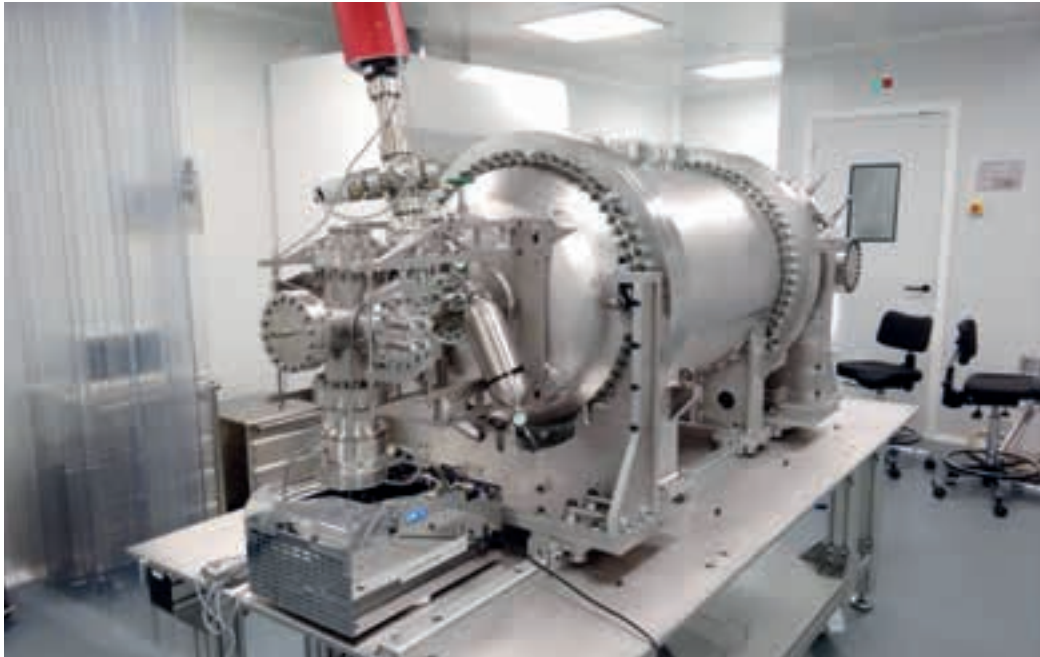
Figure 6.3: The NEW detector being assembled in the LSC clean room in 2015. The picture shows the detector seen from the Energy Plane side. The EP “cross” holds the feedthroughs (each cross side allows the extraction of 4 PMT signals) and also connects to the vacuum pump used to make vacuum in the vacuum side of the detector (in the picture the pump displays the level of vacuum achieved, 4.9 \cdot 10^{-5} mbar). The RGA is also clearly visible.
