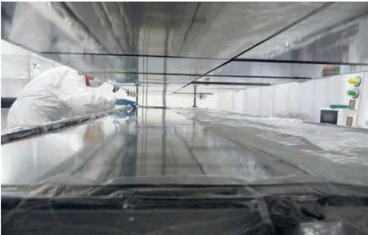
Fig. 7.1: Installation of a sample in one of the BiPo-3 modules.
