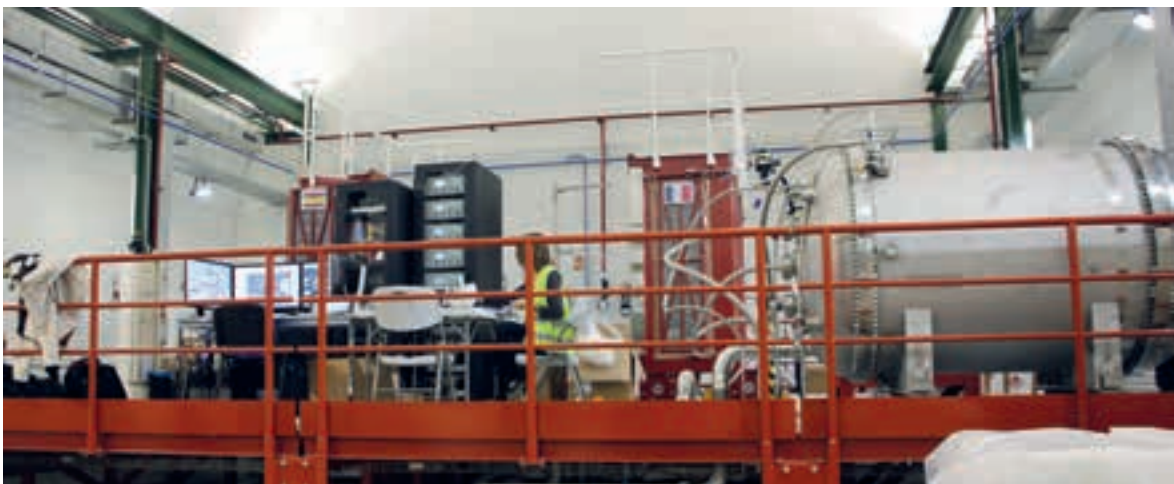
Figure 6.1: The NEXT working platform, showing the Lead Castle and the Gas system. The NEXT-100 pressure vessel (right side of picture) is used as Emergency Recovery Tank.
