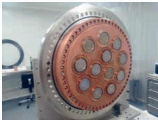
Figure 6.4: Assembly of the Energy Plane at the LSC clean room in 2015. The picture shows the end-cup plate (mother-can) with the sapphire windows already installed.
