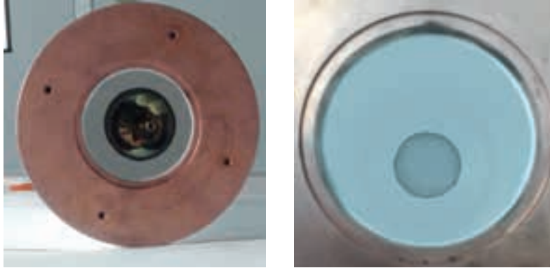
Fig. 4.5. Design considered for the first Monte Carlo evaluation of the veto effect on ANAIS 3x3 immersed in a liquid scintillator.
