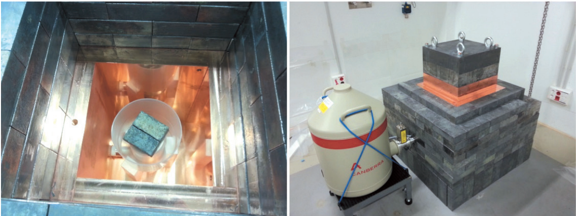
Fig. 4.5 Left: One counter while being mounted inside the copper and lead shields. Right: Opening of the shield by lifting the door
