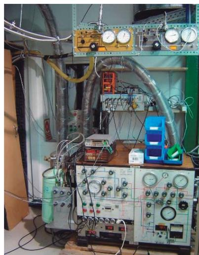
Fig. 9.4. The dilution refrigerator inside the Faraday cage with the shielding partially mounted
