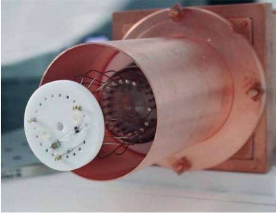
Fig. 7.2. The photomultiplier inside the copper housing, after coupling to the NaI crystal
