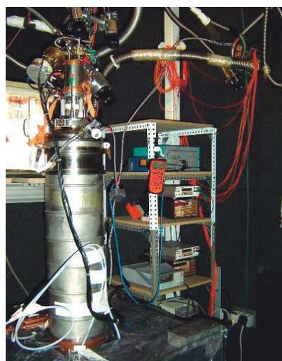
Fig. 9.3. Gas handling and pumping system for the dilution refrigerator
