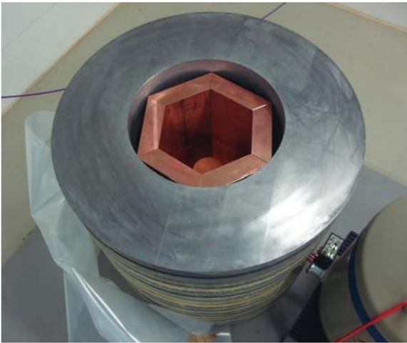
One counter while being mounted inside the copper and lead shields
