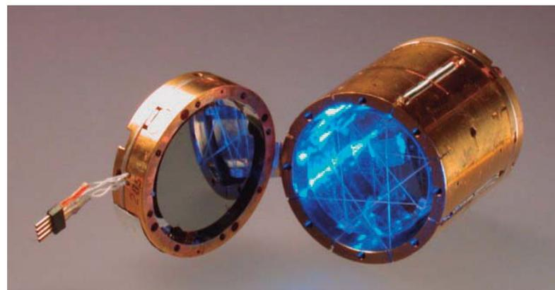
Fig. 9.1. A scintillating bolometer. The light produced in the scintillating crystal (right) is absorbed in the Ge disk (left)
