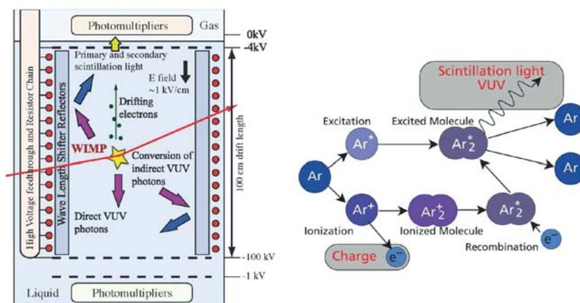
Fig. 8.1. Principles of the liquid Ar two-phase TPC
