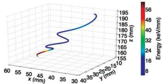
Fig. 10.3. An electron track reconstructed by NEXT-DEMO
