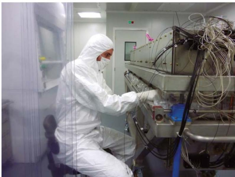
Fig. 11.2. Assembling of one of the BiPo-3 modules in the underground clean room
