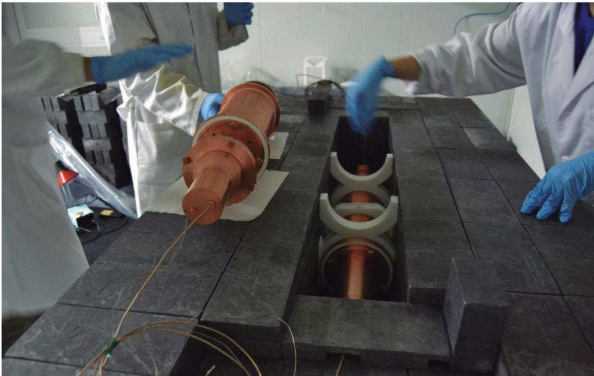
Fig. 7.1. Two NaI detectors being installed in their Cu and Pb shields
