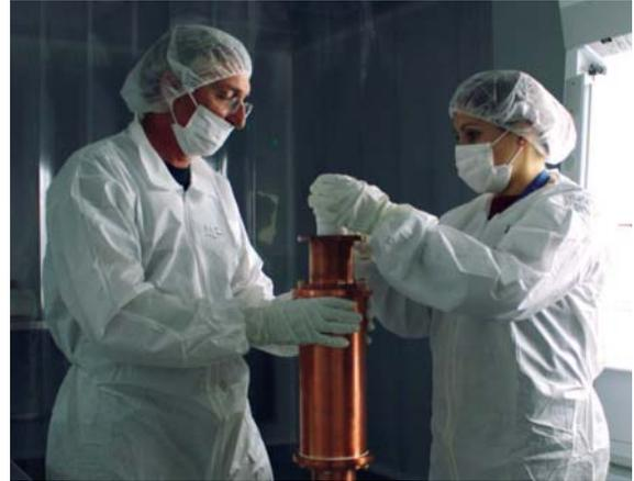
Fig. 7.3. Working on a NaI detector at LSC clean room
