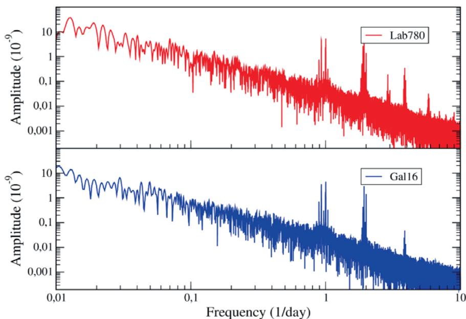
Fig. 13.5. Amplitude spectra of strain recorded by the two interferometers
