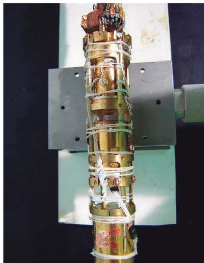
Fig. 9.2. Three scintillating bolometers mounted inside a copper frame thermally coupled to the mixing chamber of the dilution refrigerator
