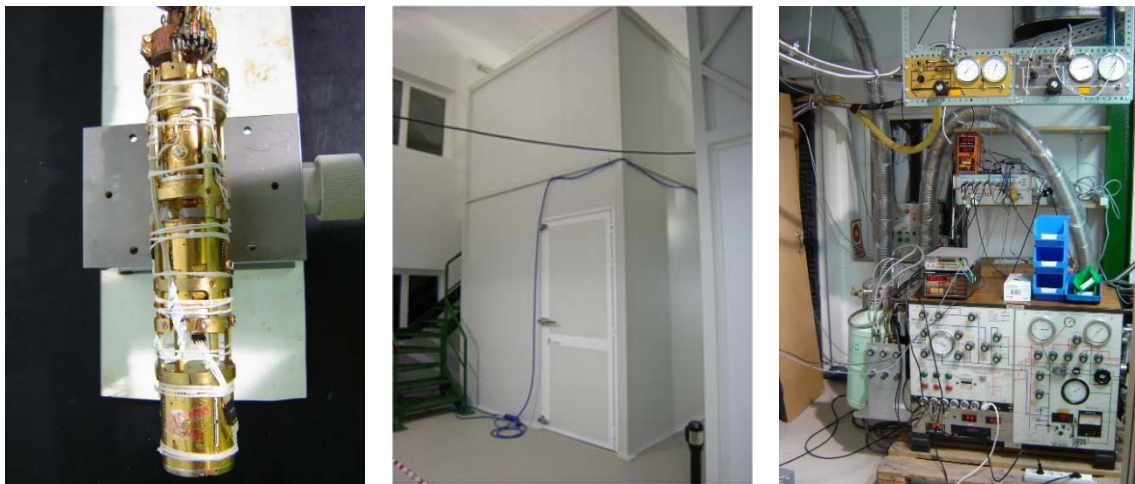
Fig. 4. Experimental set-up at Hall B of the LSC. Left: Three scintillating bolometers mounted each inside a copper frame thermally coupled to the mixing chamber of the DR. Center: Acoustically isolated Faraday cage. Left: Gas handling and pumping system for the DR.
