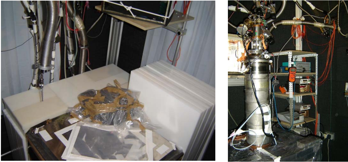
Fig. 5. Pictures of the DR at Hall B of the LSC inside the Faraday cage with the shielding partially mounted.
